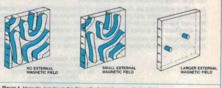
Figure 1. Magnetic domains in thin film under increasing magnetic bias field.
