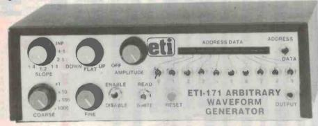
IN THE NOT too distant past when I was working with electronic test and measurement instrumentation, I was confronted with an instrument which could be programmed to create waveforms of any shape. This quite intrigued me. The applications of the device included simulation of waveforms, control signal generation and digital bit pattern generation. Instantly I saw it as the best thing since sliced bread due to its inherent flexibility and its potential for generating sound.
